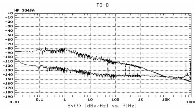
Fig.9. Spectral density of the voltage in R1-R2; the heating current noise is 6 dB higher.
