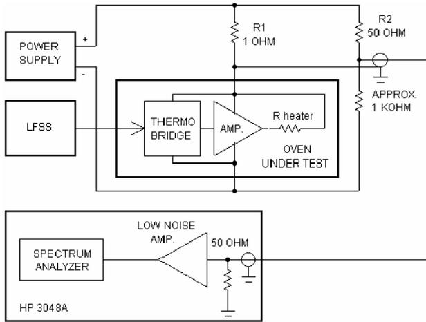
Fig. 5. Experiment test set for oven's current noise measurements.
