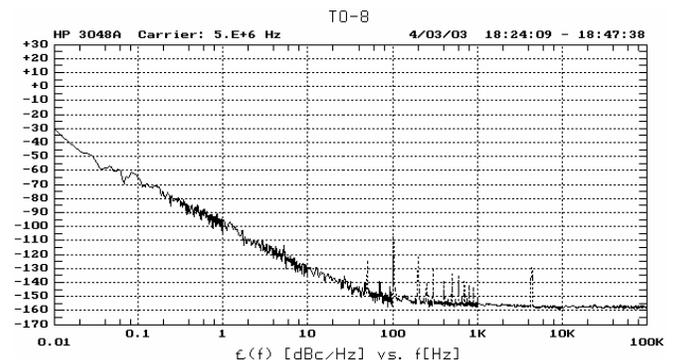
Fig. 4. Typical phase-noise behavior of two “TO-8” DOCXOs.
