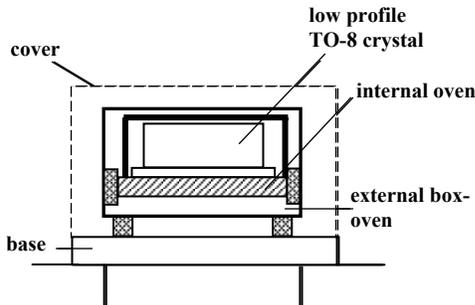
Fig.1. Schematic drawing of the “conventional” DOCXO.
