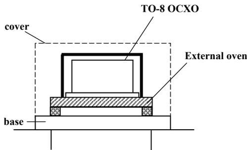
Fig. 2. Schematic drawing of the “TO-8” DOCXO.
