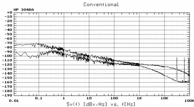
Fig. 8. Spectral density of the voltage in R1-R2; the heating current noise is 6dB higher.
