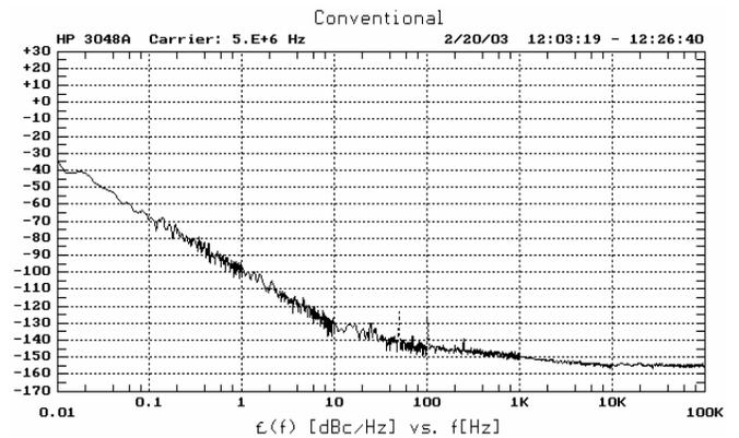
Fig. 3. Typical phase-noise behavior of two “conventional” DOCXOs.
